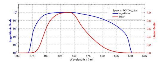
GaP blue light detector with integrated amplifier
